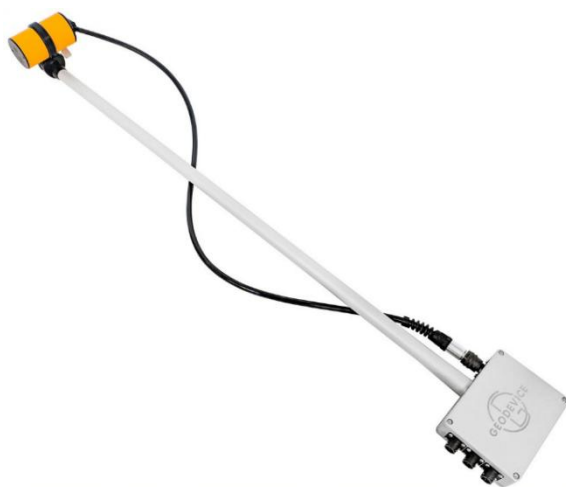
Figure 17 Overhauser sensor and OVHmag electronics unit on rod
