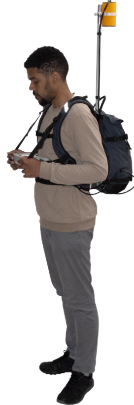
Figure 40 Vertically oriented sensor on cable
