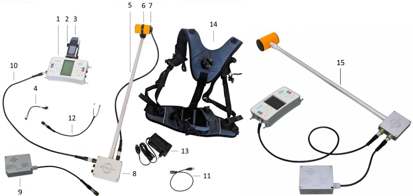
Figure 6 MaxiMag Magnetometer with sensor on cable (left) and on rod (right)
