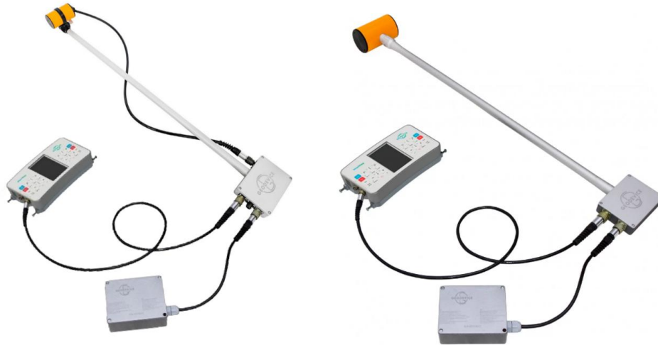
Figure 7 Small-sized Overhauser sensor on cable (left) and standard on rod (right)
