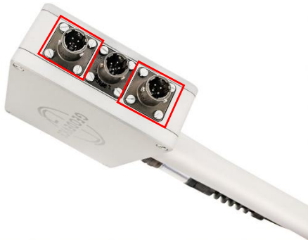
Figure 20 CAN FD + 12V connectors on the side of the electronics unit for battery connection
