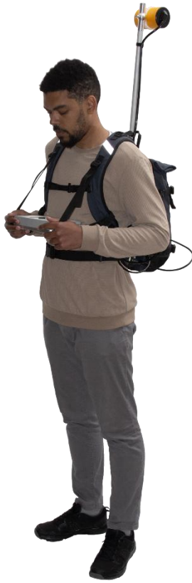
Figure 39 Horizontally oriented sensor on cable
