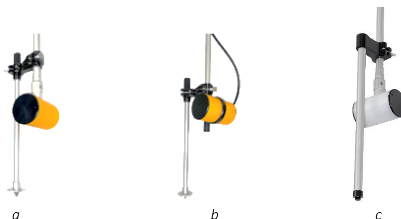
Figure 31 Mounting options for gradiometer rod to a – sensor on rod; b - sensor on cable; sensor on rod, after 2022-year model
